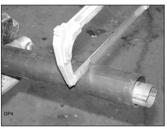
Figure 7. Cut Shield
